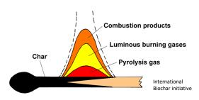
of pyrolysis products is not complete in forest fires or inefficient stoves. Pyrolysis is a source of pollutants formation (CO, aromatics, "brown carbon" in organic aerosol, etc.). Therefore, it is important to better understand pyrolysis mechanisms in order to reduce the health and environmental impact of biomass combustion.
