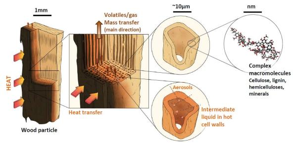
Herein, heat is brought by only one side of the particle in order to highlight the thermal gradient inside the particle and the chemical profile from char to pristine (not converted) wood. In reactor, heat is brought all around the external surface of the particle and is better conducted along the fibers' axe. The first important issue is to assess the anisotropic heat transfer inside wood particles.
